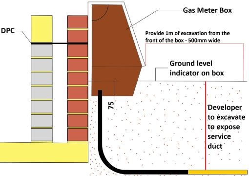
If we are installing low pressure services, meters **must not** be within 150mm of any electrical apparatus and should be 150mm away from air bricks, windows, door openings or any opening to the property. They **must not** be positioned above any drain or air brick.
