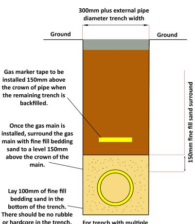
For trench with multiple utilities gas pipe must be a minimum of 250mm from all other pipes and cables
