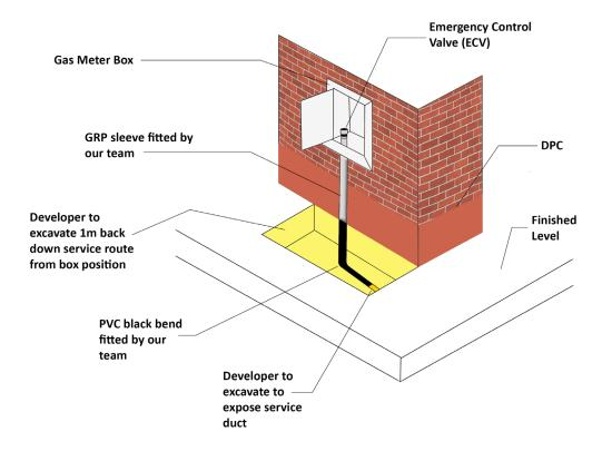
If we are installing low pressure services, meters **must not** be within 150mm of any electrical apparatus and should be 150mm away from air bricks, windows, door openings or any opening to the property. They **must** not be positioned above any drain or air brick.
